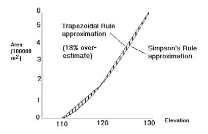
As you can see, Simpson's Rule is a better fit to the curve of the area vs elevation function.
