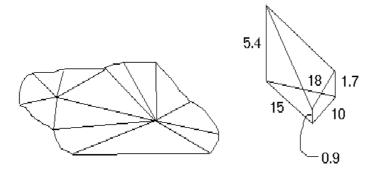
Spot levels located by tacheometry or similar. Volume calculated by multiplying areas of triangle by the average of the corner heights.
