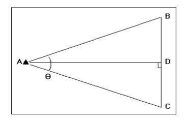
If the angle BAC ( $\Theta$ ) is known, as well as the length BC, then the distance AD can be calculated. This is the principle behind the subtense bar (an obsolete piece of surveying equipment): AD = BD/(tan Q/2)
