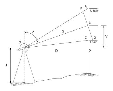
Imagine a staff inclined at B, so that it is at right angles to the line of sight. Staff intercept is then FG.
